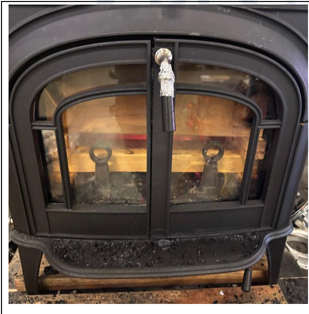
Test Fuel Loaded in Stove
