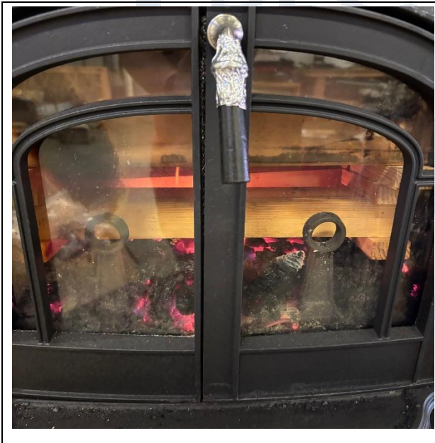
Test Fuel Loaded in Stove
