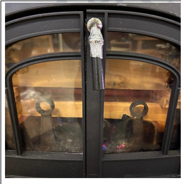
Test Fuel Loaded in Stove
