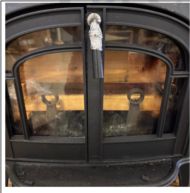
Test Fuel Loaded in Stove
