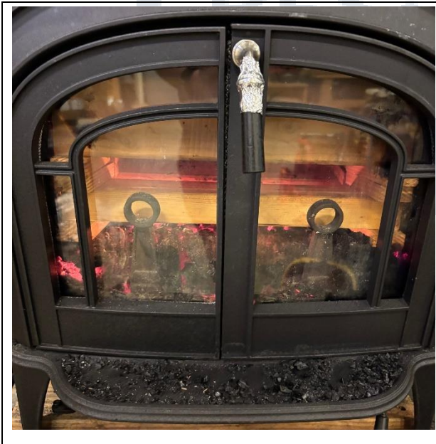
Test Fuel Loaded in Stove
